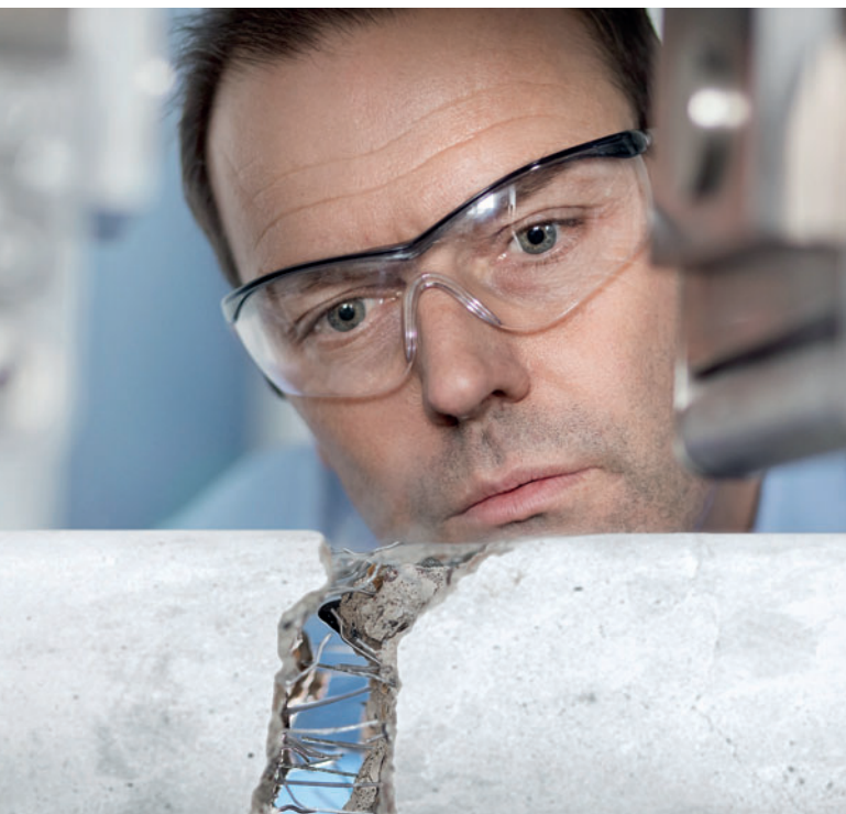
KrampeHarex internal quality control, beam test for SFRC performance
