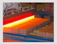
INFRARED DRYING EQUIPMENT (NIR TECHNOLOGY)
