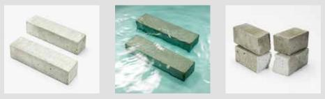
TWO SPECIMENS, THE ONE ABOVE UNTREATED, THE ONE BELOW PROTECT-TREATED, THREE STEPS: DRY – WATER BATH – AFTER
